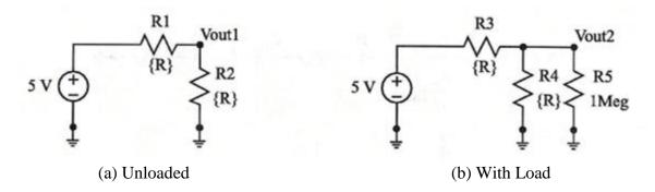
Figure 6.5: Circuits to test the loading effect of a measuring instrument having a  $1M\Omega$  input resistance.
