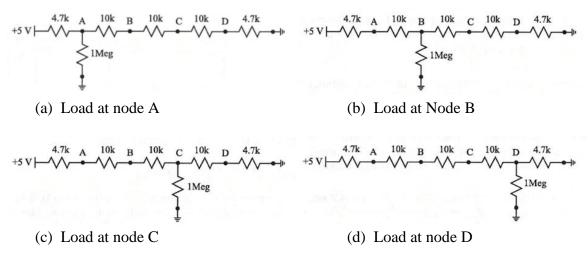
Figure 6.4: Resistor string ladder with a 1 M $\Omega$  resistor load attached at one of the nodes A through D in each diagram.
