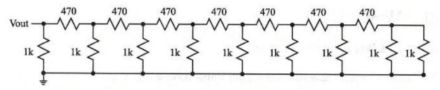
Figure 6.7: An 8-bit R - 2R ladder with all of the digital bits tied to ground.
